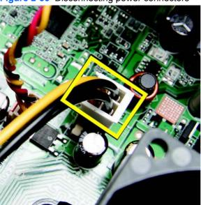
Figure 2-55 Disconnecting power connectors
